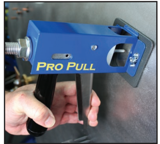
Pro Pull Dent Pulling. Position the weld tip in the bottom of the dent, weld, then squeeze the handle to initialize the pulling action.
