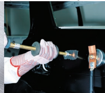
Spot hammer welding
