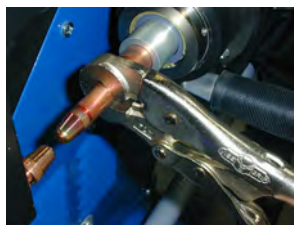
Figure 5.6a: Removing Piston Electrode
