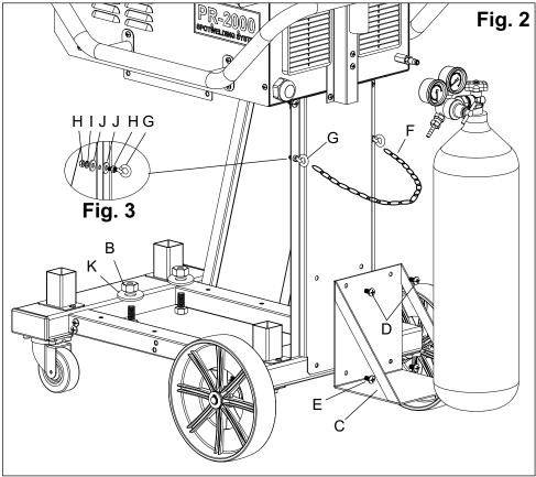
**Please NOTE:** Side Member on this drawing has been removed for viewing purposes only! **Do not** remove side member on your welder during installation.
