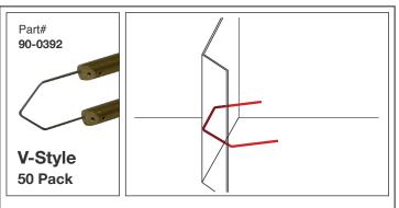
The **V-Style** staples are designed to weld inside corners (such as the inside of two overlapping plastic pieces that join at an angle).
