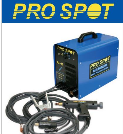
Pro Spot AL-5 Capacitor Discharge Stud Welder is designed for aluminum dent pulling but can also be used with steel studs for welding to UHSS panels with no or very little heat applied to the panels. The welder is very easy to use and is controlled by one knob to adjust duration of weld time. The welder auto detects the line voltage between 110 VAC – 240 VAC.
