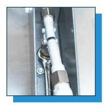
2.3 Place the open end of a 12mm (½") box wrench over the air tube release ring.
