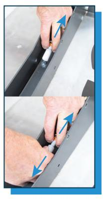
3.2 To remove the Muffler, depress the tube release ring in and pull on the Muffler at the same time.
