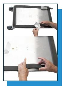
5.6 Apply the piece of the replacement gasket to the metal plate by pressing firmly.
