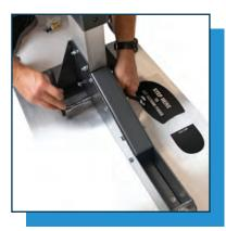
3.1 Remove venturi cover from the base plate.
