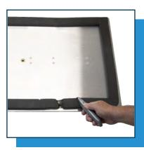
5.1 Use a razor knife to cut the piece of the gasket in two parallel lines at 45°.
