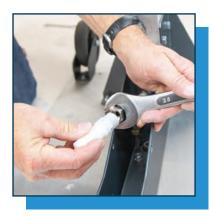
2.6 Unscrew and remove the Muffler.
