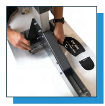
2.1 Remove venturi cover from the base plate
