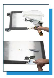
5.3 Thoroughly clean the surface with adhesive remover and scraper.
