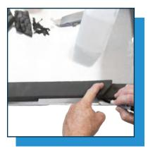
5.5 Measure a piece from spare gasket to fit into the cut area. Make sure to add at least 0.25 inch on both sides.
