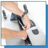
2.2 Gently lift the muffler end of the Venturi to easily access the air tube release ring on the base plate air fitting.
