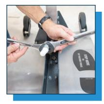
2.5 Using a 25mm wrench on the large nut, and a 21mm wrench on the Muffler hex, loosen the Muffler.
