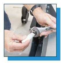
2.6 Unscrew and remove the Muffler.
