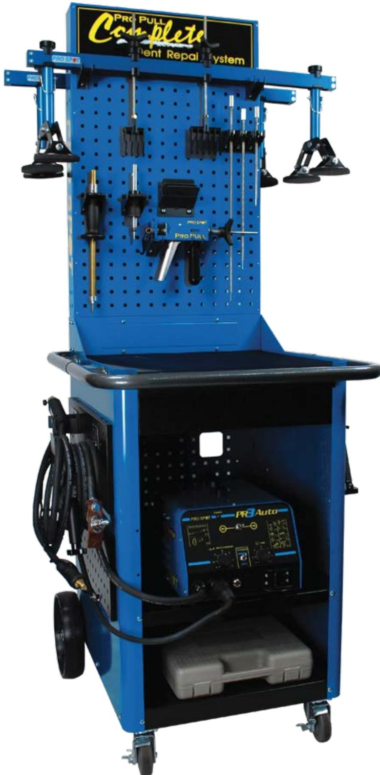
The Pro Pull Complete utilizes the all new PR-3 Auto to generate the precise, High Power/Low Weld time needed to prevent damage to the corrosion protection on the backside of the panel.
