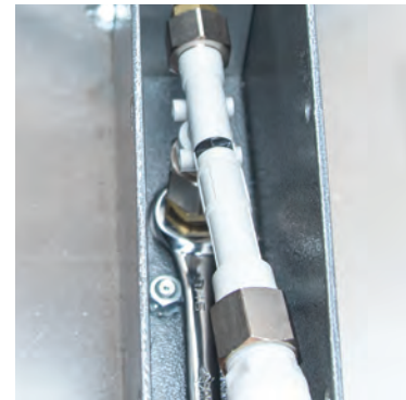
3. Place the open end of a 12mm (1/2") box wrench over the air tube release ring.
