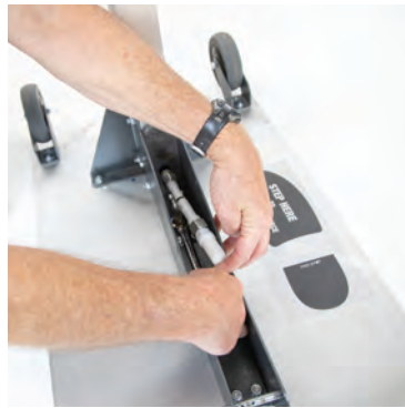
2. Gently lift the muffer end of the Venturi to easily access the air tube release ring on the base plate air fitting.
