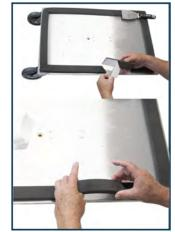
Apply the piece of the replacement gasket to the metal plate by pressing firmly.
