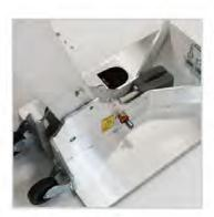
3. VERICAL COLUMN Install vertical column: metal hook on top should be facing front.
