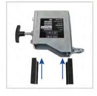
NOTE: When replacing the slider rails, place them so the edges will hold the tower edges. The sliders go between the bolts on the inside of the slider.
