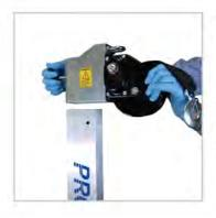
6d. Position slider rails inside of the slider and replace the winch/slider assembly on the tower. Tighten the knob on the back of the slider to secure the winch.
