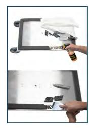
Thoroughly clean the surface with adhesive remover and scraper.
