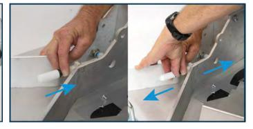
To remove the Muffler, depress the tube release ring in and pull on the Muffler at the same time.
