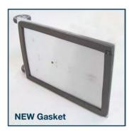
The gasket will need to be re-glued. Make sure to clean the old glue off first. We recommend 3M 4298UV adhesion promoter, or equivalent, and then spray adhesive to glue back on.
