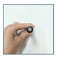
Inspect the inside of the Muffler. Look for dirt, debris or other contaminants that could clog the filter wall of the Muffler.
