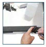
Measure a piece from spare gasket to fit into the cut area. Make sure to add at least 0.25 inch on both sides.
