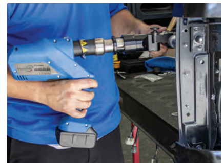
Use the Blind Rivet Adapter with the Henrob Conversion Kit
