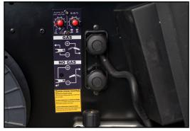
Easily change the electrode polarity for use with solid wire (electrode positive) or flux core wire (electrode negative).
