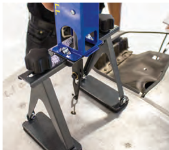
The PRO-65 provides targeted dent pulling
