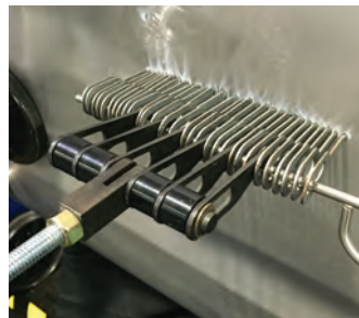
Tightly arrange keys for a more consistent pull
