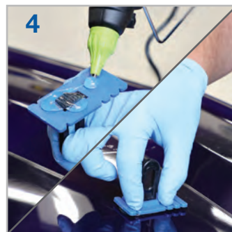
4 Apply glue to the pull tab and set it on the dent in the area you wish to pull.
