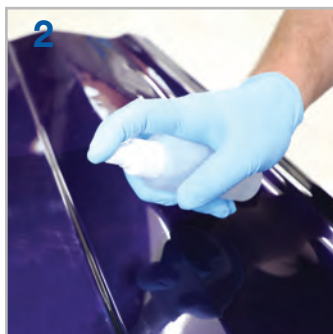
2 With 91% alcohol, clean the area you plan on repairing.
