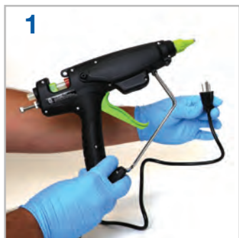
1 Plug in the glue gun and let it heat up while you prepare the dent and materials.
