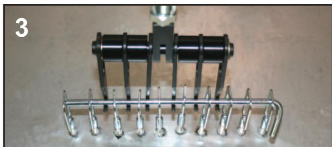
Pro Spot AL-5 Capacitor Discharge Stud Welder is designed for aluminum dent pulling but can also be used with steel studs for welding to UHSS panels with no or very little heat applied to the panels. The welder is very easy to use and is controlled by one knob to adjust duration of weld time. The welder auto detects the line voltage between 110 VAC – 240 VAC.
